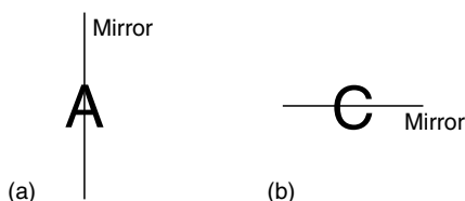
Figure 3.1 Symmetry of letters: (a) A; (b) C. The symmetry element in each case is a mirror, represented by a line
