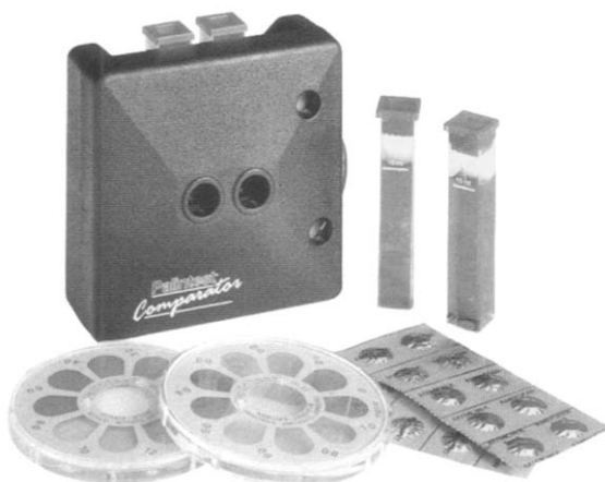
Fig. 4.1. System of discs with a comparator from Palintest company.
