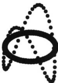
Figure 3-2. The real part of the first and second excited state wavefunctions for a particle confined to a ring of constant radius are shown.
